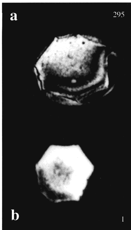
Figure 7. Gradient-echo images collected (a) at 0 °C during the swelling process of SILS and (b) at 50 °C after the polymerization reaction. xy -field of view (FOV): 11 mm; voxel resolution 86 \times 86 \times 500 \mu\text{m}^3 ; RG = 200; NE = 300; TE = 3.54 ms; TR = 1 s.
